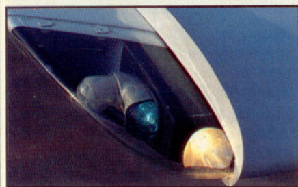
Wing-tip navigation and strobe lights (above), together with rear-facing recognition lights, give maximum visibility.
