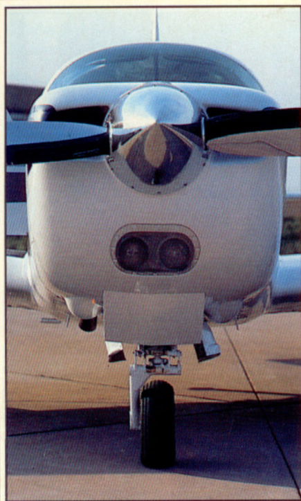
Electrically actuated single-cowl flap (above) is adjustable to any position. NACA duct (below) keeps ice, snow away from intake air.
