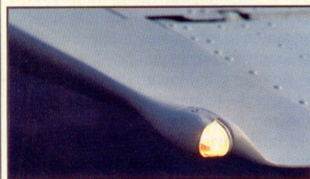
Wing-tip navigation and strobe lights (above), together with rear-facing recognition lights, give maximum visibility.
